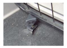
3 Now position the Dog Guard so that the slotted bracket fits around the rear seat catch. See photograph 3. When the seats are up right they hold the guard in position.
