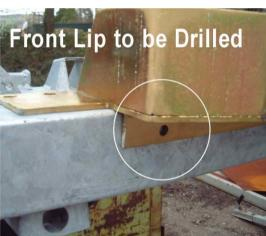
There are another 2 holes that need to be drilled. These are on top of the bumper where the winch is to be positioned. It may be necessary to enlarge the other bolt holes depending on the winch application.
