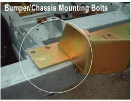
The lip, with 2 bolt holes, on the winch mount should now be in front of the bumper. Drill the bumper and bolt.
